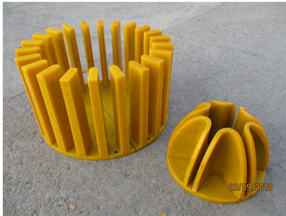
Outotec impeller and stator. Impeller dia 650
